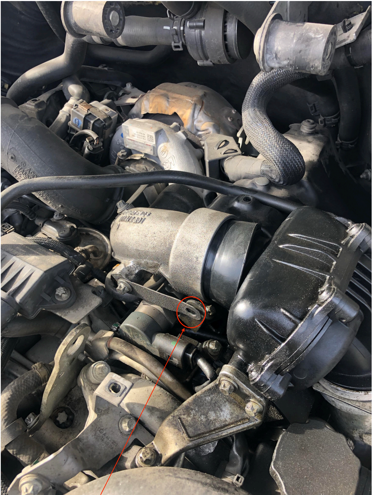
This missing bolt is common. It causes the air intake tubes to get loose and cause the engine to go into limp home.
