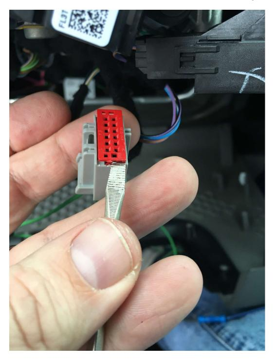
Then simple push the new terminals into the position described above. And reinstall the red retainer. Then I wrapped this two wires with Tesa tape back to the HSWM.
