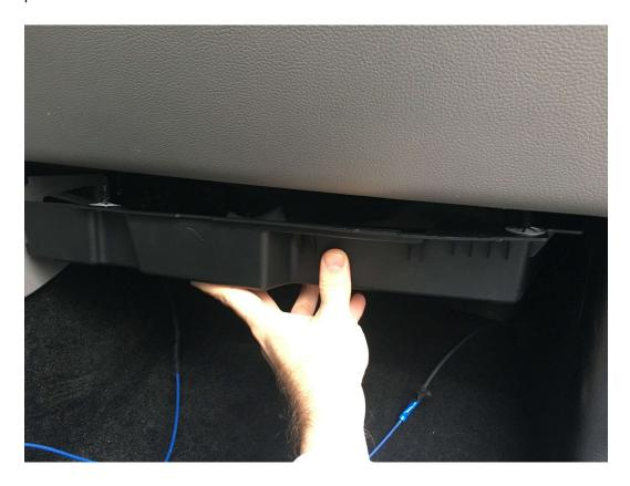
To get to the BCM there is a cover that swings open. At the back there is a place to put your fingers in and pull. Once at 90 degrees you can remove the cover by pulling towards the drivers side.
