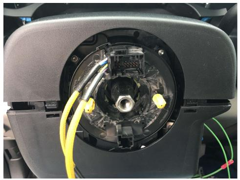
Pop up the trim that connects between the top of the shroud and instrument panel. Then the top will now be able to be removed.
