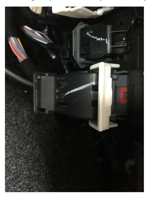
Cut tie wrap off and make sure you don't cut the wires (picture was taken with it already off). Then there is a tab where I am pointing to that you press in and push up and the top cover should come off. Then remove the red terminal retainer. I used a small screw driver on each side. You will see there is a tab that the red retainer needs to clear on both sides.
