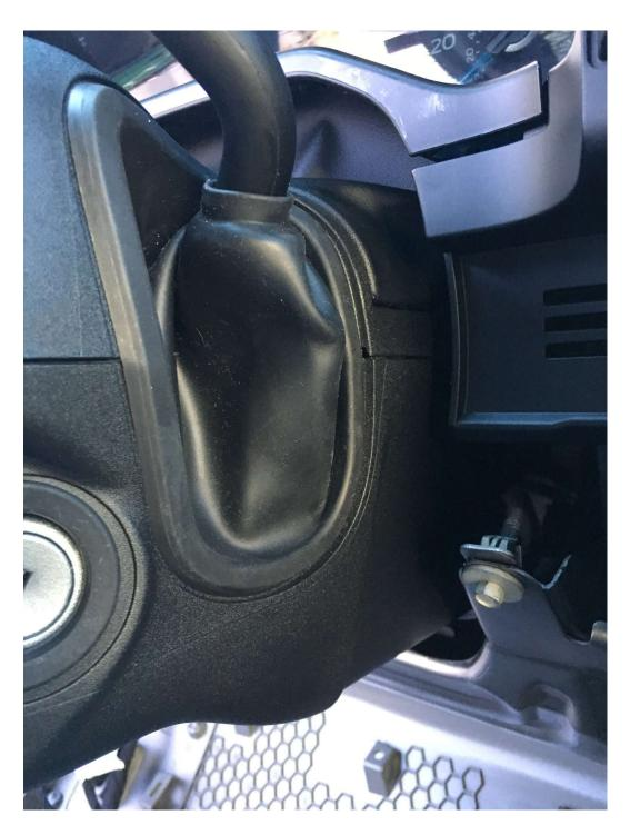
Flip up the plastic knee guard, line up clips and push into place.
