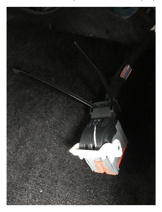
Reinstall plug to BCM by putting the connector in place and moving the locking lever towards the front of the truck. You should see the connector go closer to the BCM while doing so.
