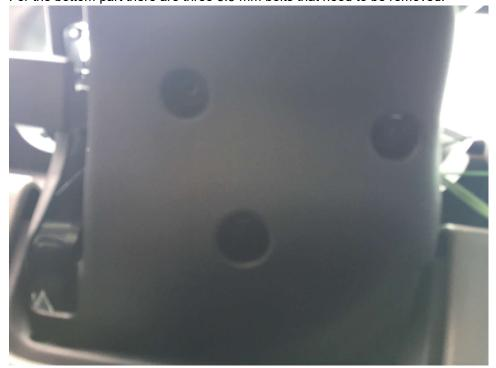
Lower the plastic where your knees would be. This is simple just have to grab onto the top on each side of the steering column to get it to lower.
