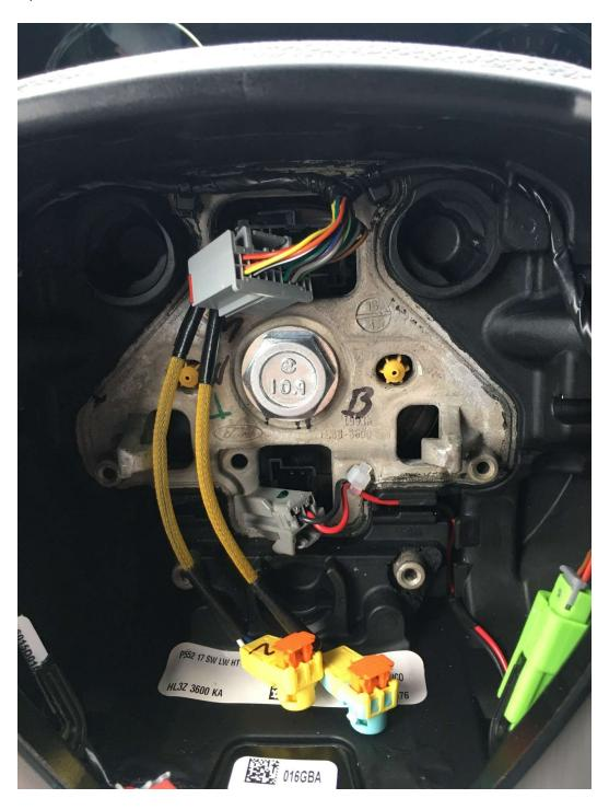
Try not to move the clock spring and put some tape on it so that it will not move. You're clock spring will not have the bottom connector. I took these pictures after already installing it.
