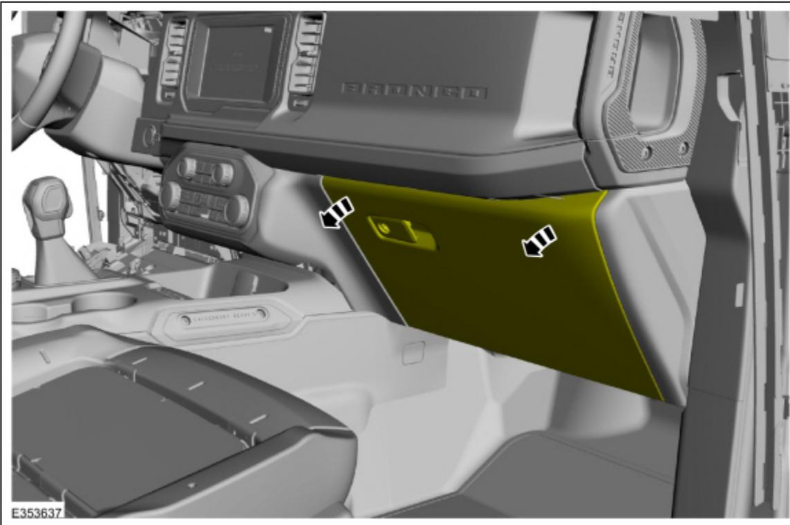
6. **NOTE:** Vehicles not equipped with a handle are equipped with a trim plate. The bolts and trim plate must be removed.
