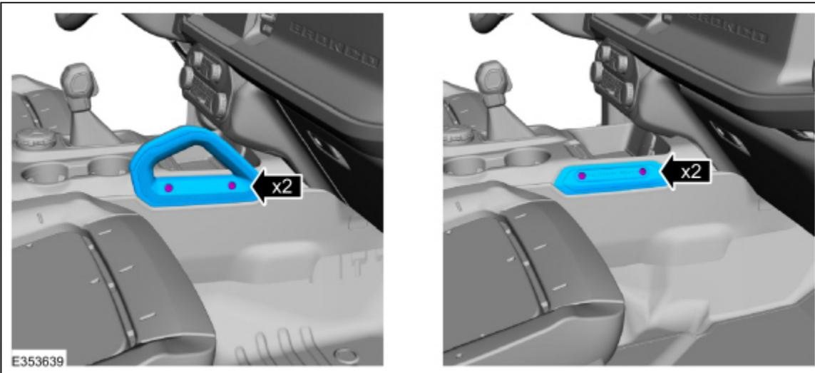
7. Remove the screws, release the retainers and remove the lower instrument panel trim panel.
