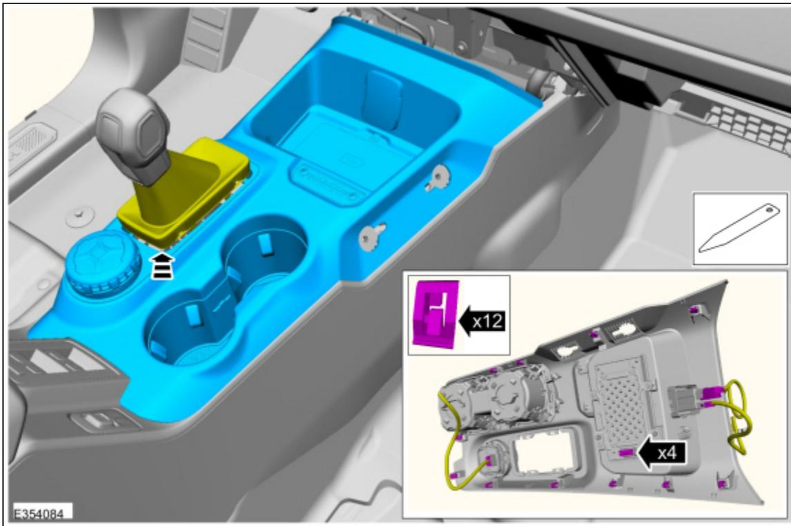
10. Remove the bolts and the console reinforcement bracket
