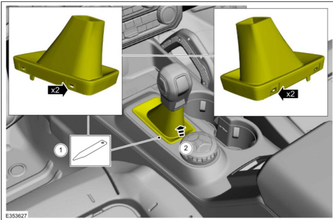
9. Release the retainers, feed the shift boot through the panel opening, and remove the floor console upper trim panel.
