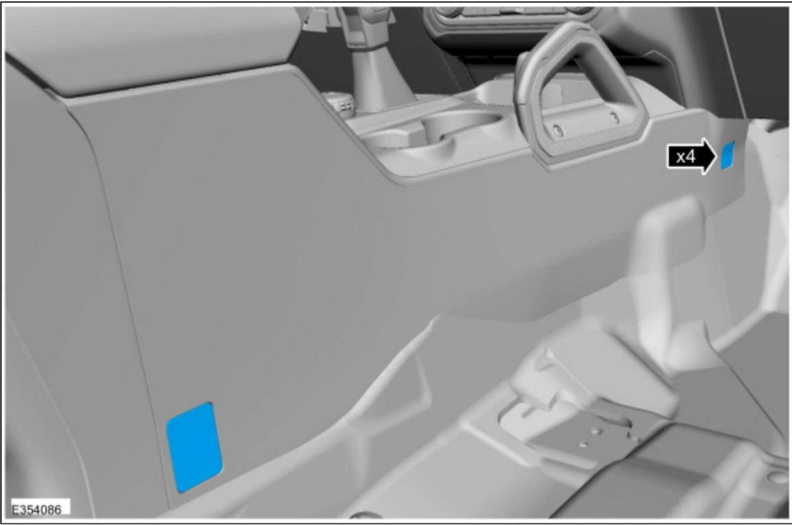
4. Release the retainers and lower the steering column opening trim panel.
