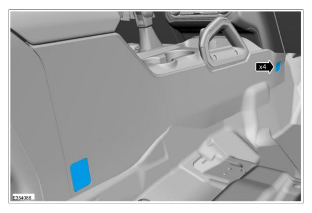
4. Release the retainers and lower the steering column opening trim panel. Use the General Equipment: Interior Trim Remover
