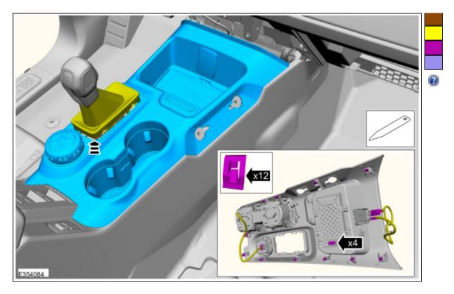
10. Remove the bolts and the console reinforcement bracket *Torque*: 22 lb.in (2.5 Nm)
