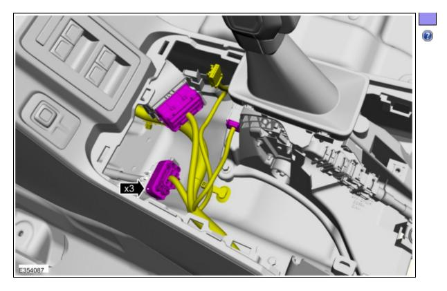
12. Remove the bolts, release the push pins and remove the floor console. *Torque*: 48 lb.in (5.4 Nm)
