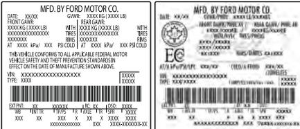
The Safety Compliance Certification label is located on the door hinge pillar, door-latch post, or the door edge that meets the door-latch post, next to the driver seating position.
