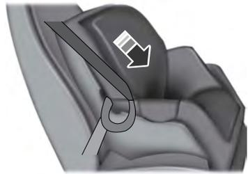
5. To put the retractor in the automatic locking mode, grasp the shoulder portion of the belt and pull downward until you pull all of the seatbelt out.
