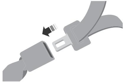
4. Insert the belt tongue into the proper buckle for that seating position until the latch engages. Make sure the tongue is latched securely by pulling on it.
