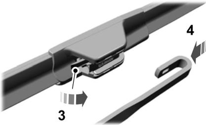
3. Press the wiper blade secondary locking clip.
