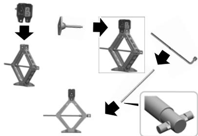
9. Do not use the extension block when you are changing a flat tire on the rear of the vehicle. Assemble the jack handle using the extensions as shown to operate the jack when placing under the rear axle.
