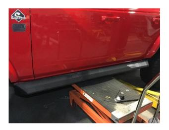
7. Using a lift table or a friend, lift the sliders into position and fasten the two body mount nuts onto the studs. Leave loose for now.
