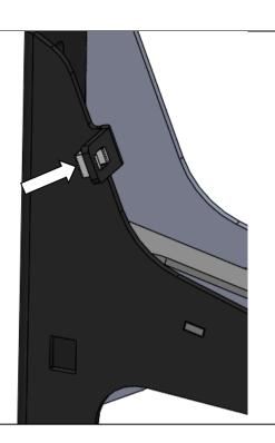
6. Insert M6 cage nut into rear mount of left slider.
