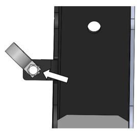
11. Using P-Clip provided, attach the wiring harness with an M6x25 bolt and washer to the rear mount so that it can't rub
