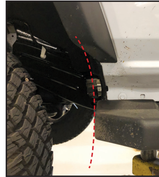
Running board sits too far forward into the wheel well
