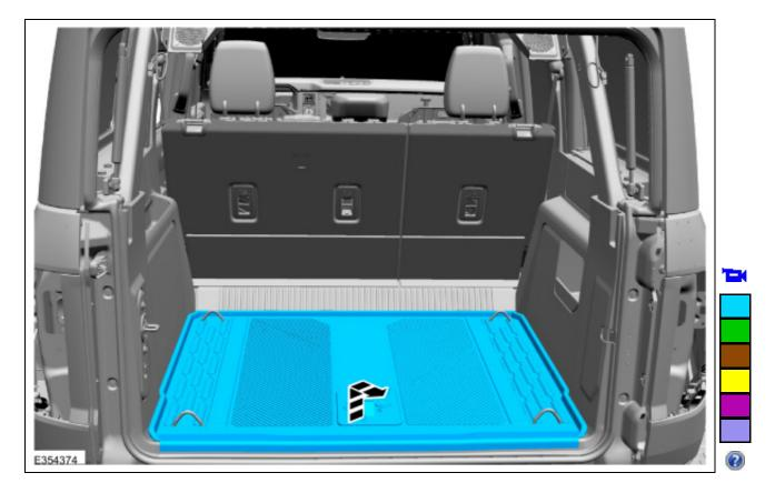
3. Release the clips and remove the loadspace scuff plate trim panel. Use the General Equipment: Interior Trim Remover
