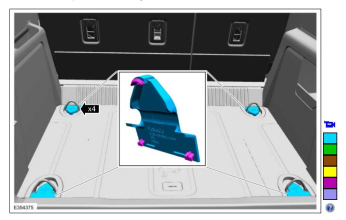
5. Remove the bolts and the load compartment floor covering tie downs.
