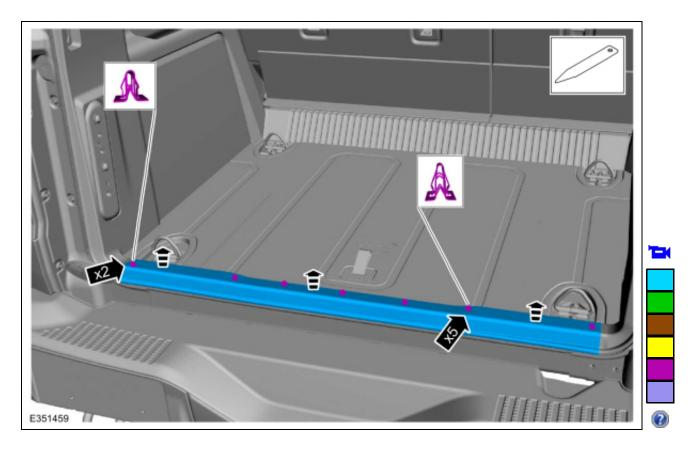
4. Remove the load compartment floor covering tie down covers.
