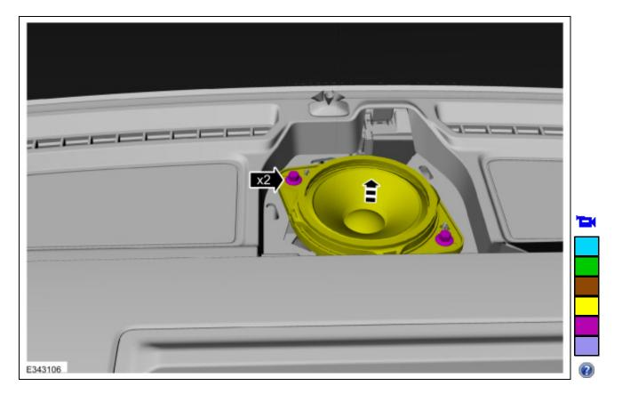
3. Disconnect the electrical connector and remove the instrument panel center speaker.
