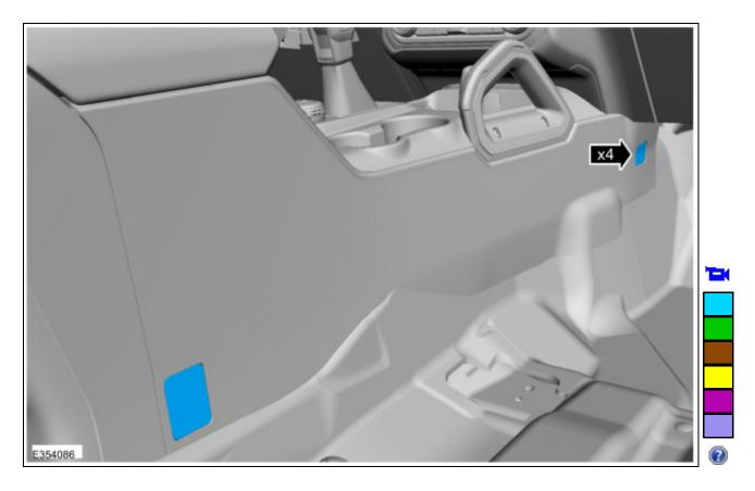
4. Release the retainers and lower the steering column opening trim panel. Use the General Equipment: Interior Trim Remover
