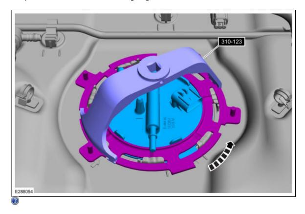
6. NOTICE: Take extra care not to damage the fuel tank level sensor and float arm.
