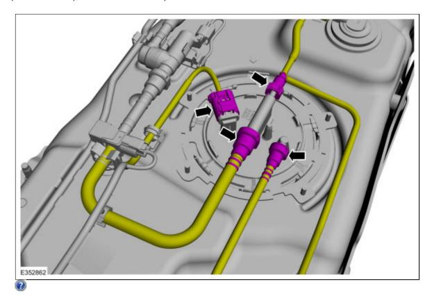
9. **NOTE:** Note the position of the fuel pump and sender unit for installation.
