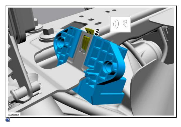
2. Connect the fuel pump driver module electrical connector.
