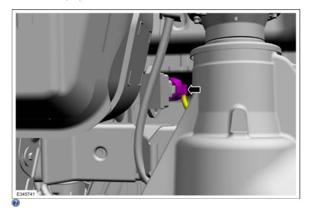
4. Release the fuel pump driver module retaining tab, then remove the fuel pump driver module from the bracket.
