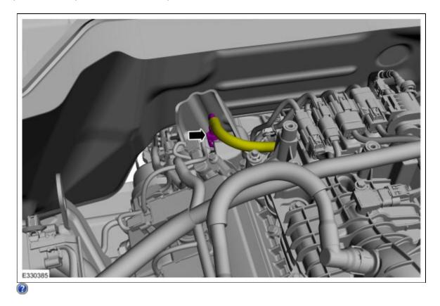
4. Install the Fuel Pressure Test Kit between the fuel supply line and the high pressure pump.
