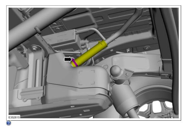
6. NOTICE: Make sure the open end of the hose is secured above the fluid level in the reservoir
