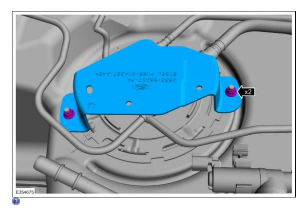
4. Disconnect the quick release couplings and remove the fuel tank pressure sensor and tube assembly.
