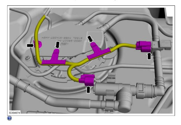
3. Remove the nuts and fuel pump sender unit shield. *Torque*: 80 lb.in (9 Nm)
