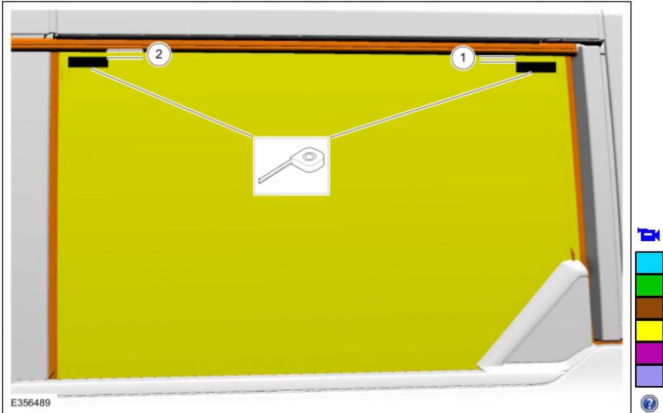
7. Subtract the distance of the marks on the tape at both locations from the previously recorded measurements in step 4.
