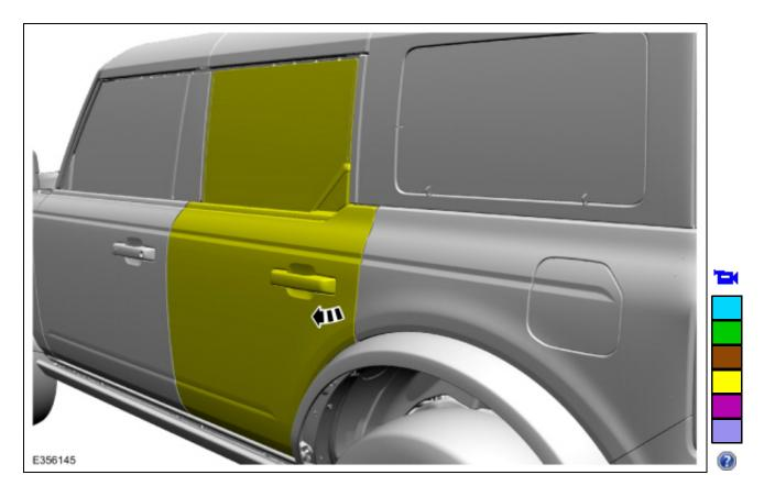
Measure the distance of the marks on the tape at both locations to the top edge of the rear door glass at the specified locations.
