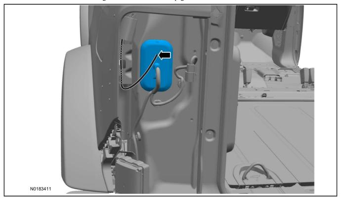
23. Seal the LH rear tail lamp grommet around wiring using Motorcraft® TA-29 Silicone Sealant or equivalent.
