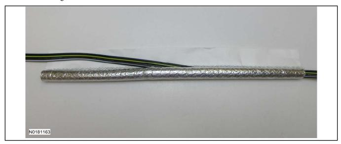
39. Remove adhesive strip backing and secure the protective heat sleeve around the 4 flat ribbon trailer wire harness.
