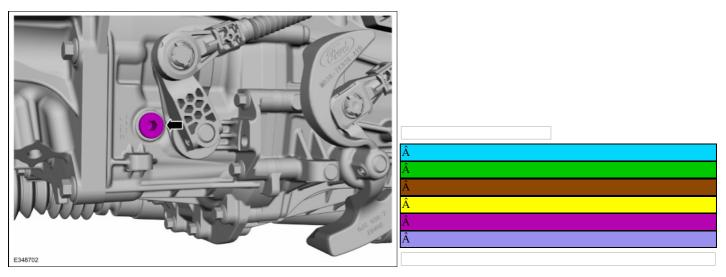
3. **NOTE:** The minimum fluid level should be no more then 3mm below the transmission fluid fill hole.
