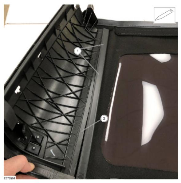
7. Center the plastic strip on the D-pillar with the plastic strip on the rear window so they sit directly on top of each other. (Figure 3)
