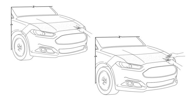
For "fingers" along the edges of the film, promptly spray the Tack solution into the finger and squeegee to the edge with a hard card wrapped with a Microfiber towel. The Microfiber towel helps with fingers along the edges by absorbing the tack solution as it is pushed out the edge of the film.
