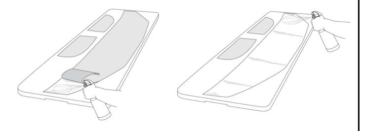
Next, spray mounting solution generously on the area in which Paint Protection Film will be applied. Gently position the film on the surface to be protected while identifying an alignment point such as the center, an emblem or a corner on the surface. For the Side Fender, using the headlight and Upper body panel are generally the best alignment points. This will be the starting point of the wet out.
