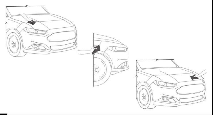
If you notice debris under the film, wet your fingers and gently lift the film from the closest edge and flush with mounting solution. Use your finger to remove the debris from the film. Once the debris is removed, re-wet the film and surface and squeegee the film back in place.
