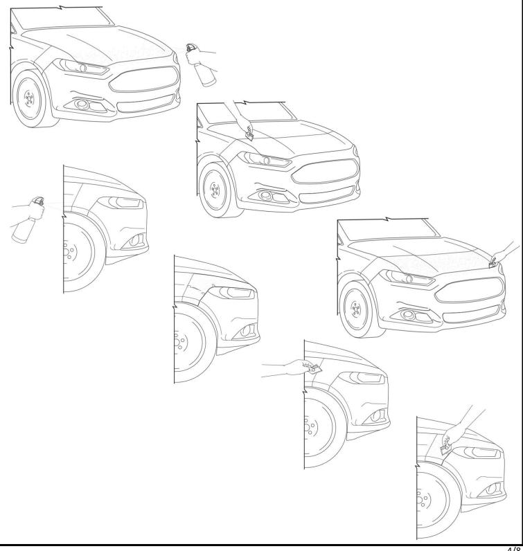
Stretch the film as necessary to align along the edges. Precut patterns account for most "fingers" in the design, so when stretching to align edges, most "fingers" will lay flat on the surface. "Fingers" are localized gaps in the film in aera of high contour. Continue to squeegee out the aid solution towards the edges as you stretch and align the film on the surface.
