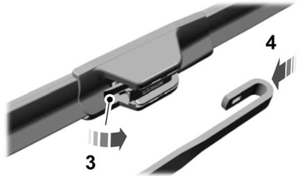
3. Press the wiper blade secondary locking clip.
