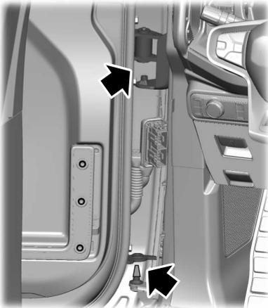
9. With the help of another person, lower the door onto the body hinges, aligning the upper door portion to the upper body pin and the lower door portion to the alignment pin.
