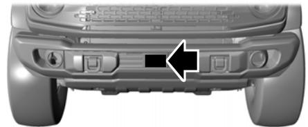
The radar sensor is in the lower grille.
