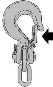
If the trailer safety chain hook has a latch, make sure to fully close the latch.
