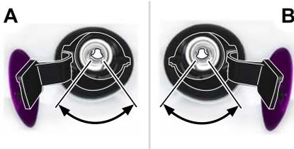
5. Operate the fuel pump nozzle within the area shown. Refer to A for left hand drive or B for right hand drive.
