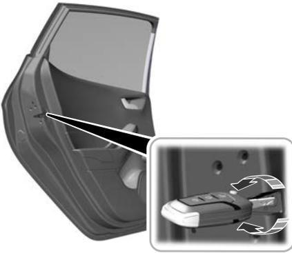
A child safety lock is on the rear edge of each rear door. Switch the child safety lock separately on each door.
