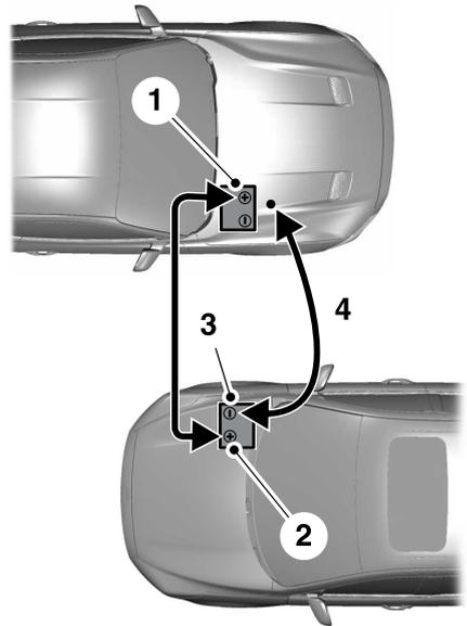
1. Pull the red rubber boot backward. Connect the positive (+) jumper cable to the positive (+) terminal of the discharged battery.
