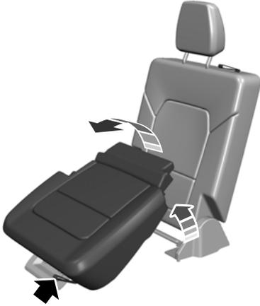
1. Pull the strap at the front of the seat cushion. Then, flip the seat cushion up to the vertical position.
