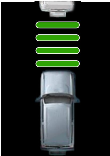
The selected gap appears in the instrument cluster display as shown by the bars in the image.
