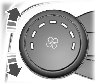
Turn the blower motor control counterclockwise for a lower blower setting.
