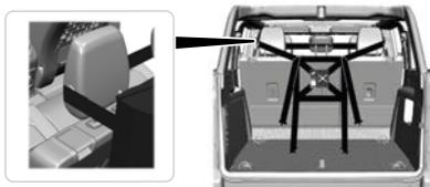
6. Place the narrow strap loop over all the rear headrests and tighten until snug.
