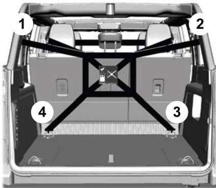
5. Attach upper straps 1 and 2 to the eyebolts. Attach lower straps 3 and 4 to the forward cargo rings.
