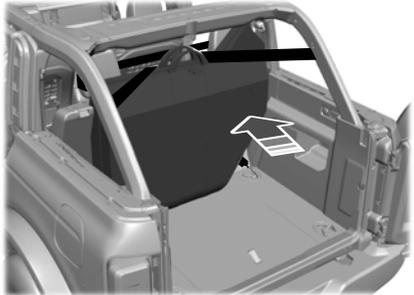
4. Zip the bag fully closed and gently place the door in the cargo area. Avoid contacting the rear pillars, speakers, striker, and trim. For soft tops, take care to avoid contacting the prop rod.
