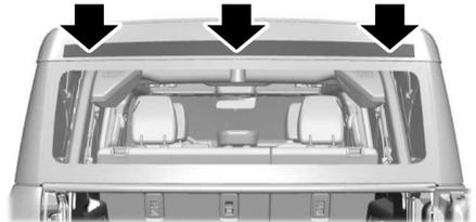
6. After installing the rear window, press along the top of the window to secure the Velcro strips.
