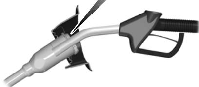
3. Insert the fuel pump nozzle up to the first notch. Keep the fuel pump nozzle resting on the fuel tank filler pipe.
