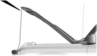
3. Open the hood and support it with the hood strut.
