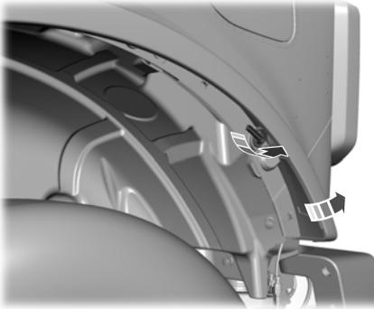
2. Loosen the quarter-turn fastener on the rearmost fender flare.
