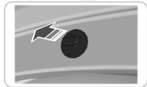
2. Pull outward on the fender flare with your hands to unseat the 5 push pin clips from the sheet metal.
