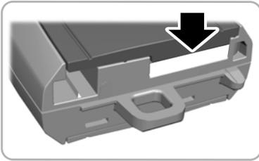
2. Twist a thin coin under the tab hidden behind the key blade head to remove the battery cover.
