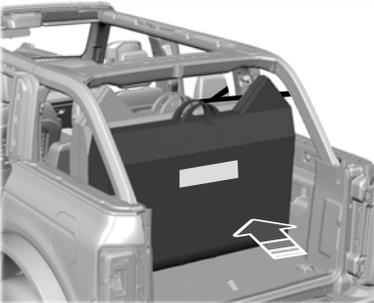
4. Zip the bag fully closed and gently place the door in the cargo area. Avoid contacting the rear pillars, speakers, striker, and trim. For soft tops, take care to avoid contacting the prop rod.
