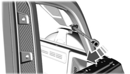
2. Use the ratchet tool provided in the kit to assist in tightening the eyebolts. The eyebolts should rest in the groove of the handle. Using the tool as a lever, apply force until fully tightened.
