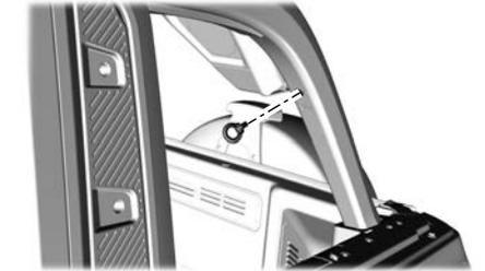
1. Install the eyebolts located in the Ford onboard storage kit into the rear cargo area pillars.
