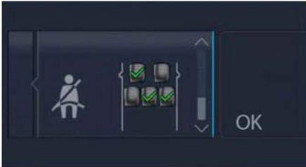
This lamp illuminates when you switch the ignition on, identifying the number of seating positions with fastened buckles. It illuminates again when a seating position changes from unfastened to fastened.
