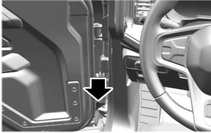
9. Locate the tool pouch and use the hex tool to remove the lower hinge bolt.
