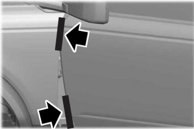
5. Locate the fender and door protectors in the tool pouch. Install one over the fender edge near the upper door hinge and the other on the door edge near the bottom door hinge.
