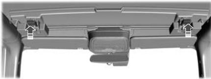
1. Unlatch the two latches in the headliner.
