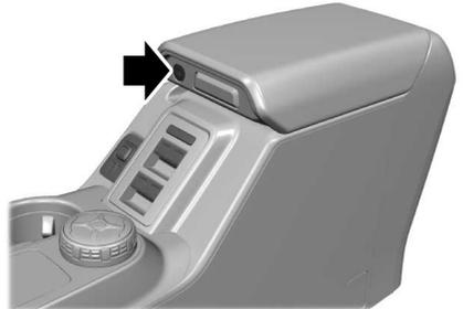
You can lock the center console using the key.
