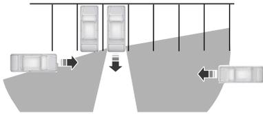
The sensor on the left-hand side is only partially obstructed and zone coverage on the right-hand side is maximized.
