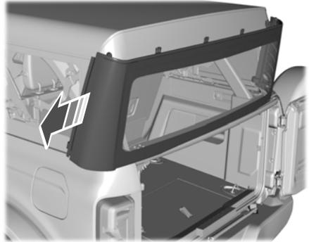
4. Slide the bottom out of the slot left or right to remove.
