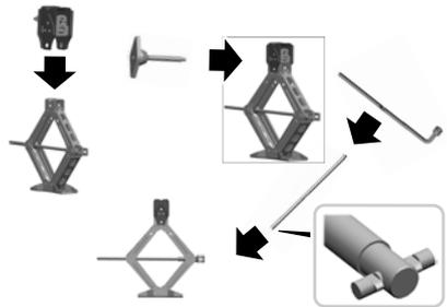
9. Do not use the extension block when you are changing a flat tire on the rear of the vehicle. Assemble the jack handle using the extensions as shown to operate the jack when placing under the rear axle.
