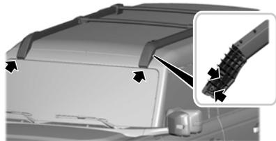
3. Using the provided T30 tool, remove the front roof rack fasteners.
