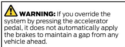
When you press the accelerator pedal, you override the set speed and gap distance.
