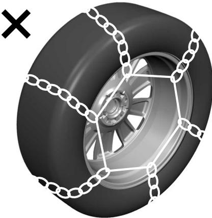
Use snow chains that fit against the sidewall of the tire to prevent the chains from touching the wheel rims or suspension, see following illustration above.
