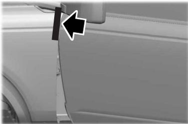
5. Locate the fender protector in the tool pouch and install it over the fender edge near the top door hinge.
