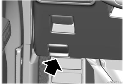
1. Pull the hood release handle under the left-hand side of the instrument panel.
