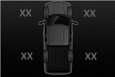
Using the information display arrow keys navigate to the truck info section where you can view the tire pressures.
