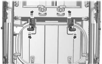
1. Pull and hold the spring-loaded slide.
