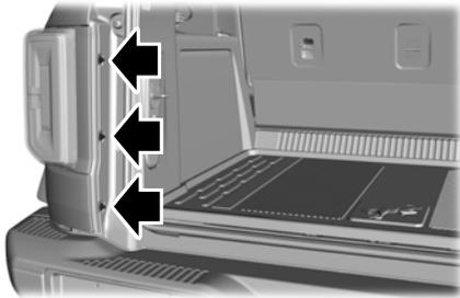
4. Remove the three pushpins from inside the trim panel.
