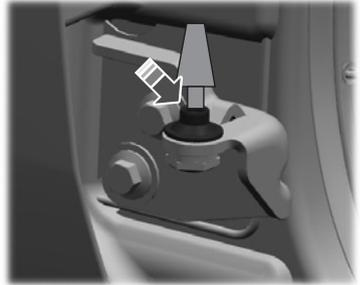
6. Locate the lower bodyside hinge and install alignment pin.
