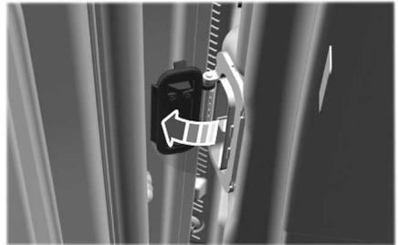
15. Insert the door harness into the connector.
