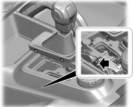
1. Insert a screwdriver between the shifter boot material and trim ring to access the retainer tabs from the top panel trim ring.
