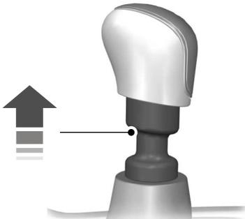
**Note:** You can only move the gearshift lever to reverse (R) by raising the collar below the gearshift knob up before shifting to reverse. This is a lockout feature which protects the transmission from accidentally engaging reverse (R) when intending to select first (1).
