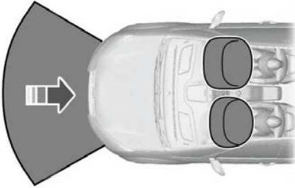
The driver and front passenger airbags deploy during significant frontal and near frontal crashes.
