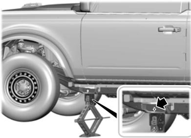
11. Use the rear axle tube for the rear jacking point.
