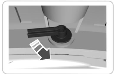
1. Unlock the five quarter turn clips by turning the clips counterclockwise.
