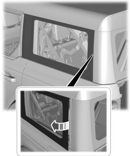
1. Release the rear edge of the panel by pulling the fabric out of the slot.
