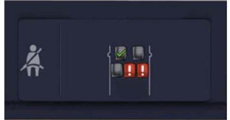
This warning displays if an occupant unfastens the rear seatbelt buckle or it becomes unfastened.
