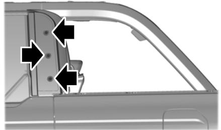
Remove the three fasteners to the soft top trim piece on each side of your vehicle using the provided head driver and ratchet.
