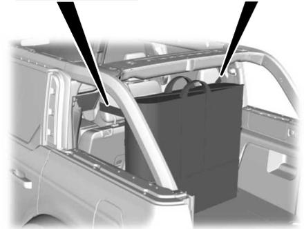
2. Secure the upper roof bag strap around the rear seat headrests. Adjust the tension on the strap until it is snug.
