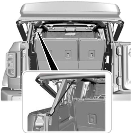
3. Lift the rear of the soft top and support it with the soft top strut.
