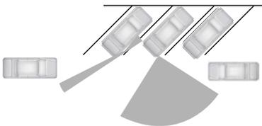
Zone coverage also decreases when parking at narrow angles. The sensor on the left-hand side is mostly obstructed and zone coverage on that side is severely reduced.
