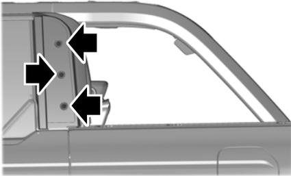
Secure the three fasteners to the soft top trim piece on each side of your vehicle using the provided head driver and ratchet.
