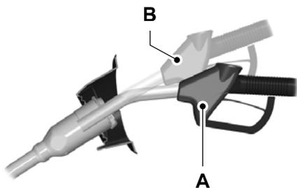
4. Hold the fuel pump nozzle in position A when refueling. Holding the fuel pump nozzle in position B can affect the flow of fuel and shut off the fuel pump nozzle before the fuel tank is full.
