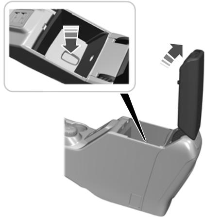
1. Place the first programmed remote in the backup slot inside the center console. With your foot off the brake pedal, press and release the push button ignition switch.
