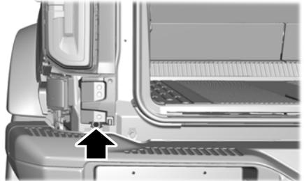
6. Remove the lower retaining bolt from the inside trim piece. Pull on the lower part of the trim piece to disengage the upper retaining clips.
