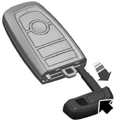
1. Push the release button and pull the key blade out.
