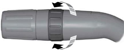
Rotate the control to the top or bottom position and hold it to operate the rear window washer.
