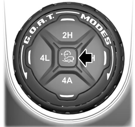
**Note:** If your vehicle is equipped with trail one pedal drive, this will activate trail one pedal drive if you are in four wheel drive high or four wheel drive low mode, until you set a speed for trail control.
