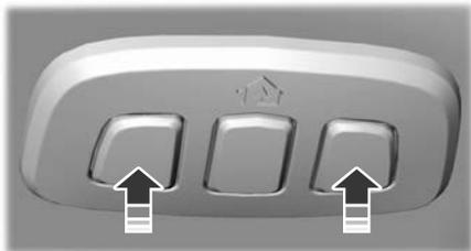
1. Press and hold the outer two function buttons simultaneously for approximately 10 seconds until the indicator light above the buttons flashes rapidly.
