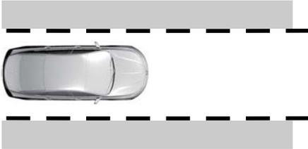
When in alert mode, the lane keeping system alerts you by vibrating the steering wheel. The intensity of the vibration is set through the lane keeping system menu.
