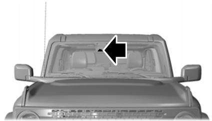
The camera is mounted on the windshield behind the interior mirror.
