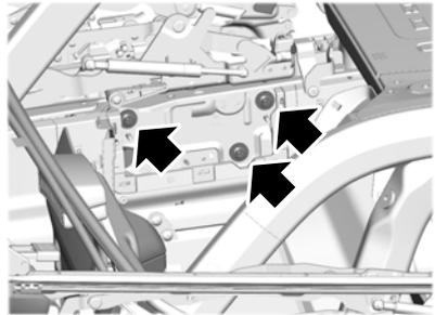
2. Remove the three fasteners on each side in the rear cargo area using the provided head driver and ratchet.
