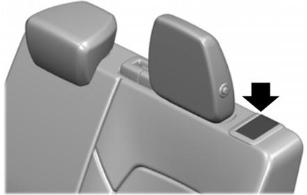
Pull the lever up to fold the seat backrest fully forward.
