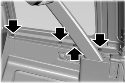
10. Remove the four fasteners on each side of your vehicle that secure the rear roof panel to the vehicle using the provided head driver and ratchet.
