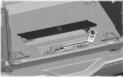
Lift the strap to access the under floor storage in the luggage compartment.
