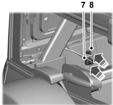
7. Secure the wiring harness to the body side by plugging it into the receptacle and pushing up on the locking tab.
