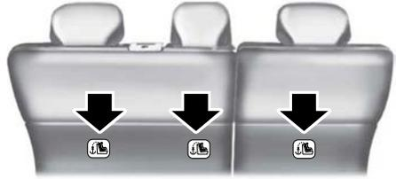
2. Locate the correct anchor behind the gap cover for the selected seating position.
