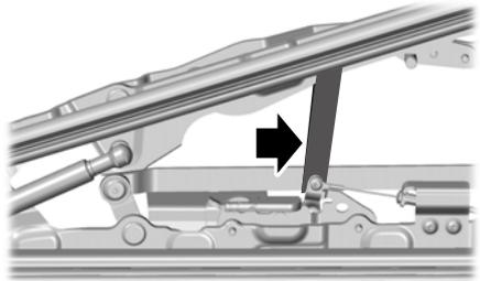
3. Attach the provided straps if you are off-road driving or driving on rough roads.
