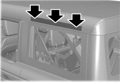
7. After installing the rear quarter windows, press along the top of the window to secure the Velcro strips.
