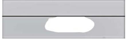
4. On the wall or screen, observe a light pattern with a distinct horizontal edge toward the right. If this edge is not at the horizontal reference line, adjust the beam so the edge is at the same height as the horizontal reference line.
