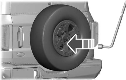
**Note:** Do not lay the wheel's face down on the ground, as there is a risk of scratching or marring the wheel if laid down on an uneven surface.
