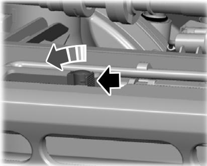
2. Release the hood latch by pushing the secondary release lever to your left-hand side.
