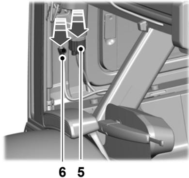
5. Push the tab inward when pulling down to disconnect and remove the wiring harness.
