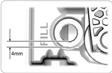
Transmission fill level is 0.16 in (4 mm) from oil fill plug.
