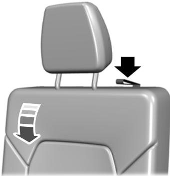
2. Pull the strap on the top of the seat backrest to fold it forward.
