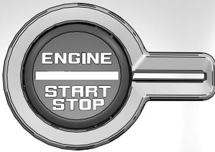
1. Press and hold the push button ignition switch until the engine stops, or press it three times within two seconds.
