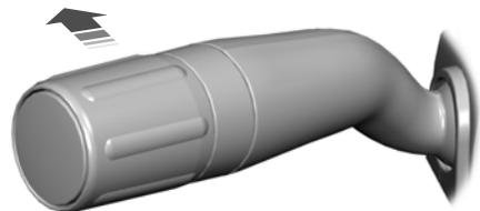
Push the lever away from you to switch the high beams on.
