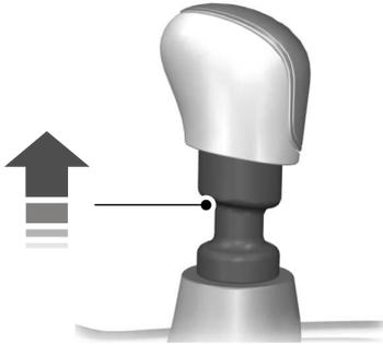
**Note:** You can only move the gearshift lever to crawler (C) by raising the collar below the gearshift knob up before shifting to crawler. This is a lockout feature which protects the transmission from accidentally engaging crawler (C) when intending to select second (2).
