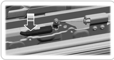
3. Press down the handle on the driver side of your vehicle to unlatch the soft top. Lift and rotate the soft top rearward, making sure to keep your hands and fingers free of the mechanism.
