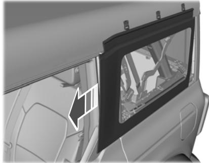
4. Slide the bottom panel forward out of the slot to remove.
