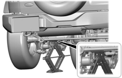
**Note:** Only use the jack on the specified jacking points and as close to the affected wheel as possible.
