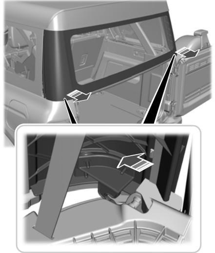
1. Pull the bottom corners of the backlight rearward to disengage the clip.
