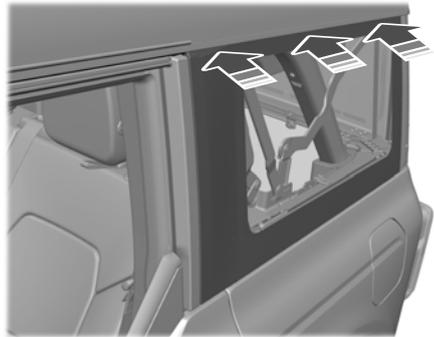
6. When installing the rear quarter windows, make sure the window is tucked under the tension cable.
