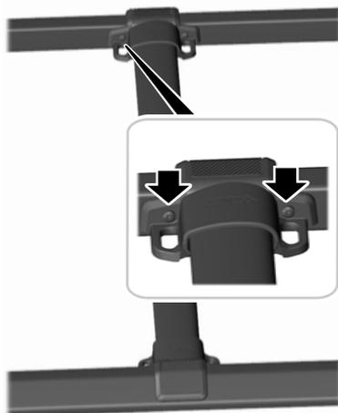
**Note:** The rear crossbar is part of the clamping system. If you removed the crossbar you must install it first for proper attachment to the hard top.
