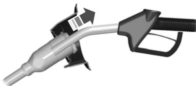
6. When the pump shuts off, wait five seconds, then raise the fuel pump nozzle and slowly remove it.
