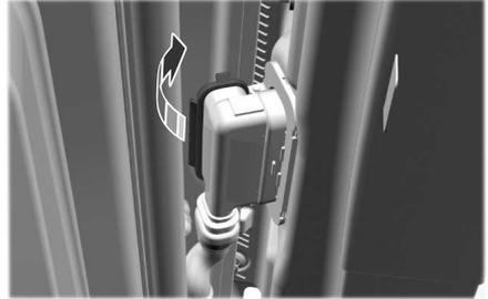
6. To release the door harness connector, open the connector door. Pull the connector straight out.
