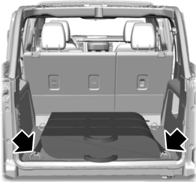
1. Install the loops through the two D-rings and secure the panels.
