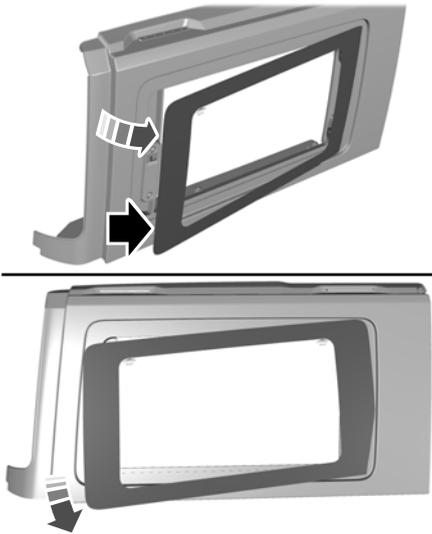
2. Rotate the quarter window while pulling down to separate the glass from the frame.
