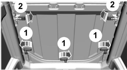
1. Turn the three L-shaped latches on the center roof panel, unlocking them from the rear roof panel.
