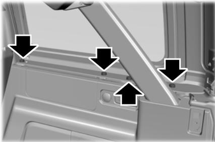
9. Remove the four fasteners on each side of your vehicle that secure the rear roof panel to the vehicle using the provided head driver and ratchet.
