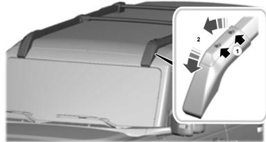
1. Using the provided T30 tool, remove the front roof rack cover fasteners.
