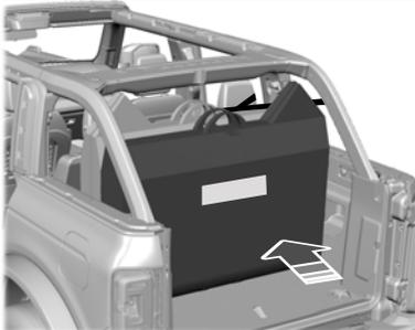
4. Zip the bag fully closed and gently place the door in the cargo area. Avoid contacting the rear pillars, speakers, striker, and trim.
