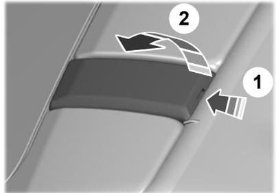
1. To remove, press the button on the rear of the cover and rotate forward.
