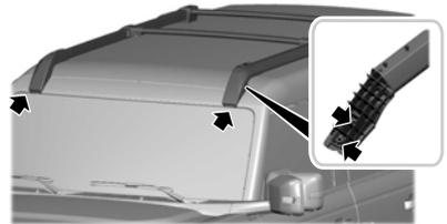
4. Position the roof rack on the vehicle.
