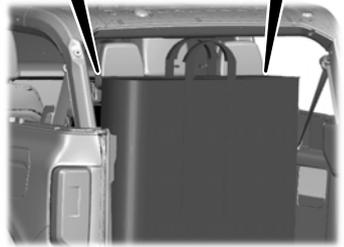
6. Secure the lower bag hooks to the forward cargo rings.
