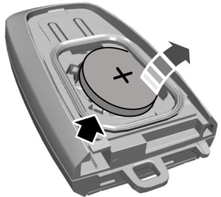
3. Insert a screwdriver, and carefully remove the battery.
