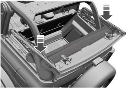
4. Press down on the driver side and passenger side of the soft top to fully secure it.
