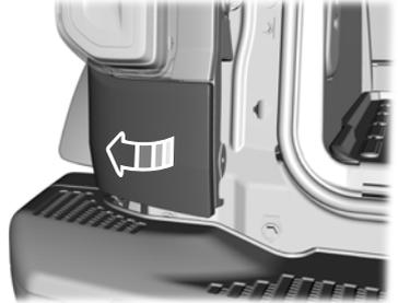
5. Remove the lower trim piece by disengaging the retaining tabs. Pull from the inside edge first, then pull from the outside edge.
