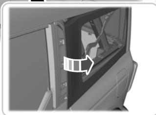
3. Release the front edge of the panel by pulling the fabric out of the slot to remove.
