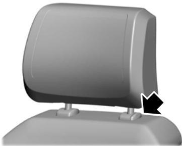
1. Pull up the head restraint until it reaches the highest adjustment position.
