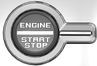
1. Press and hold the push button ignition switch until the engine stops, or press it three times within two seconds.
