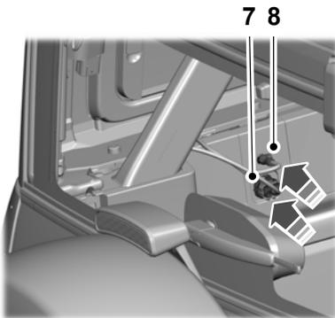
7. Secure the wiring harness to the body side by plugging it into the receptacle and pushing up on the locking tab.
