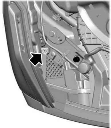
5. Locate the vertical adjuster on each headlamp. Use a #2 Phillips screwdriver to turn the adjuster either counterclockwise or clockwise in order to adjust the vertical aim of the headlamp.
