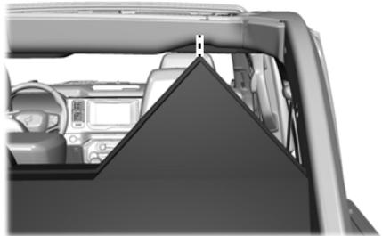
7. Secure the door bag to the retention harness with the clip.
