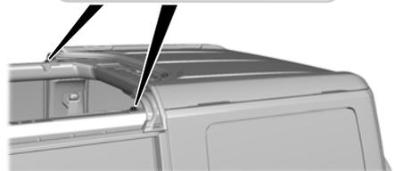
9. Remove the two fasteners that secure the rear roof panel at the C-pillar using the provided head driver and ratchet.
