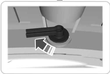
2. Lock the five quarter turn clips by turning the clips clockwise.
